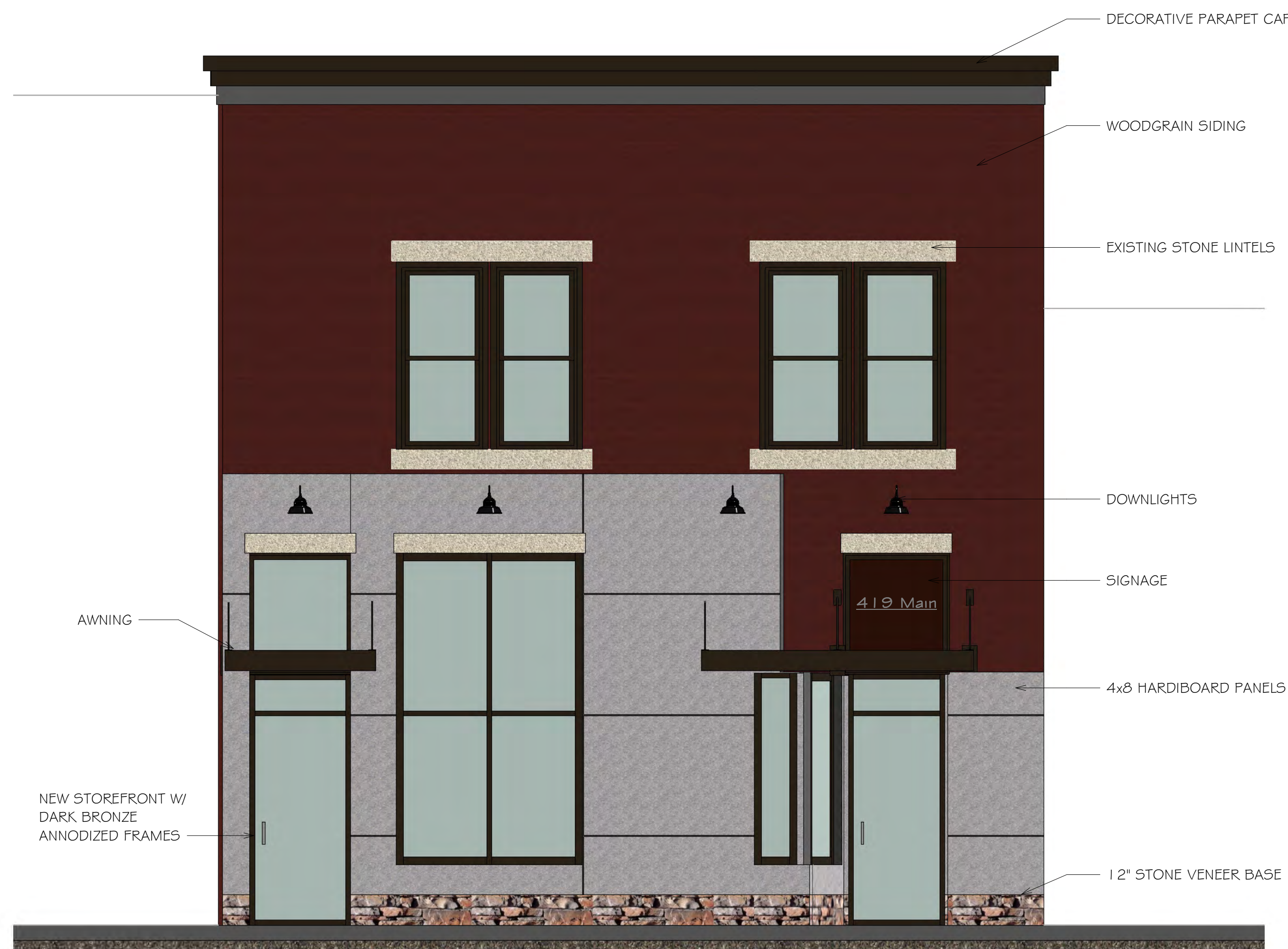
① Front Elevation 3/8" = 1'-0"
