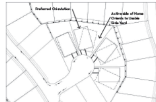
BUILDING ENVELOPE ORIENTATION
