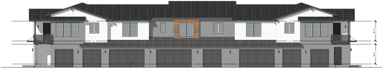
2 8-PLEX FRONT ELEVATION A-03 SCALE: 1/4" = 1'-0"
