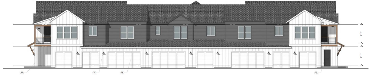
2 8-PLEX FRONT ELEVATION SCALE: 1/4" = 1'-0"
