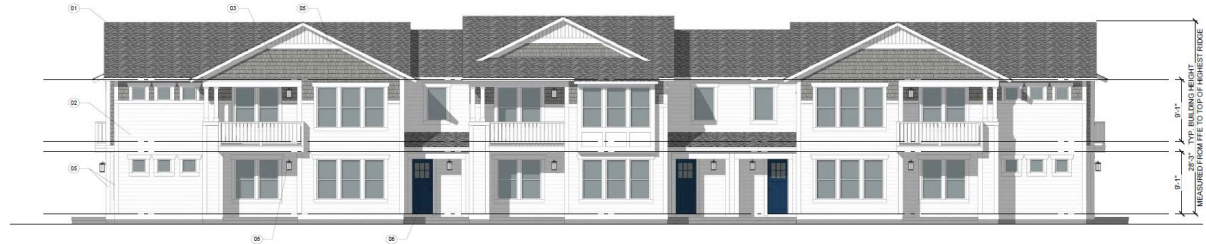
1 8-PLEX FRONT ELEVATION SCALE: 1/4" = 1'-0"
