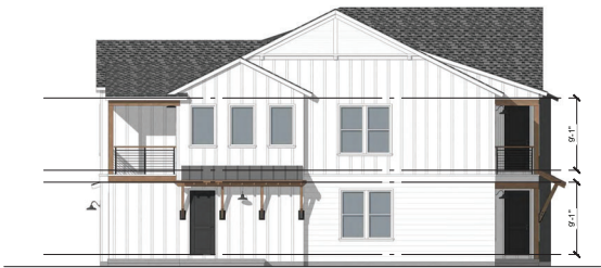
3 8-PLEX LEFT ELEVATION A-01 SCALE: 1/4" = 1'-0"
