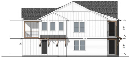
3 8-PLEX LEFT ELEVATION SCALE: 1/4" = 1'-0"
