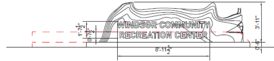
EXISTING SIGNAGE - LEFT ELEVATION SCALE: 1/4" = 1'-0"
