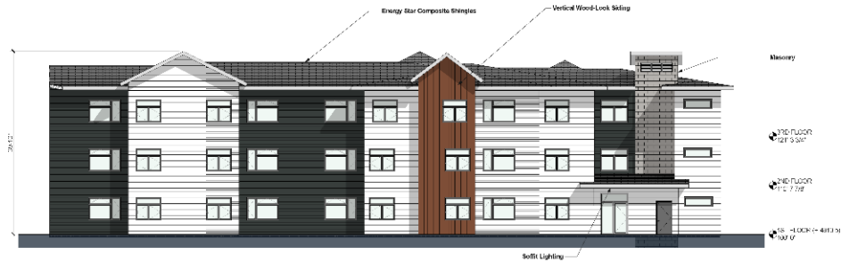
1 Elevation: Phase 1 - North View SCALE: 1" = 10'
