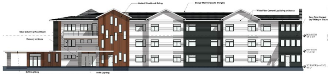
Elevation: Phase 1 - West View (Front) SCALE: 1" = 8'
