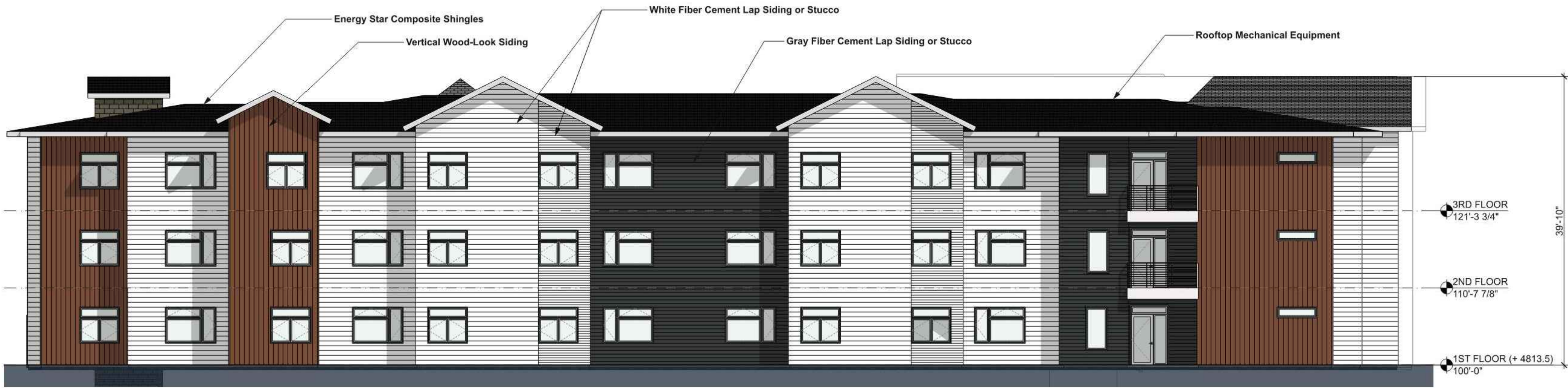
3 Elevation : Phase 1 - South View SCALE: 1" = 10'
